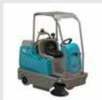
Increase safety and effective operation in the most severe environments with an optional **FOPs certified overhead guard.**
